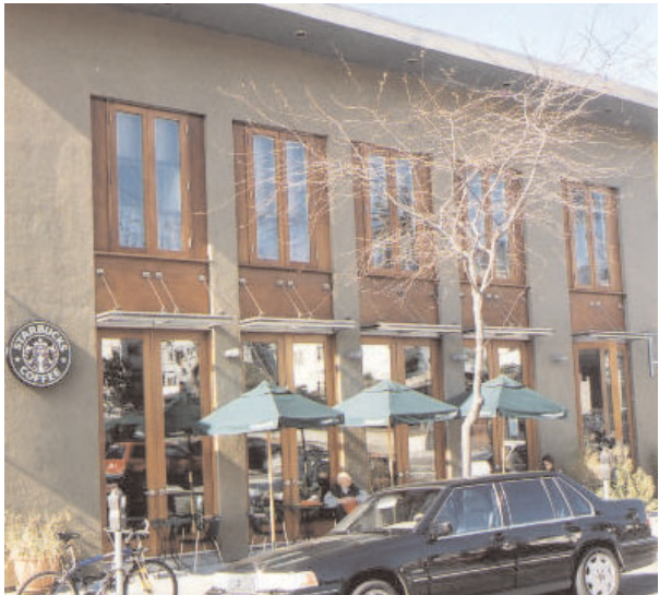
Upper-floor windows should be smaller than storefront windows on the ground floor.
