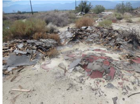
ASPHALT ROOFING, ROOF FELT, AND ROOF TAR DUMPED NEAR THE CENTER OF THE PROPERTY
