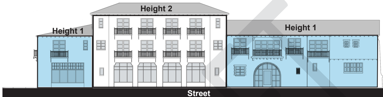
FIGURE 17.20.2XX.7 OPTION 1 STANDARDS VERTICAL MODULATION THREE FLOOR BUILDINGS
