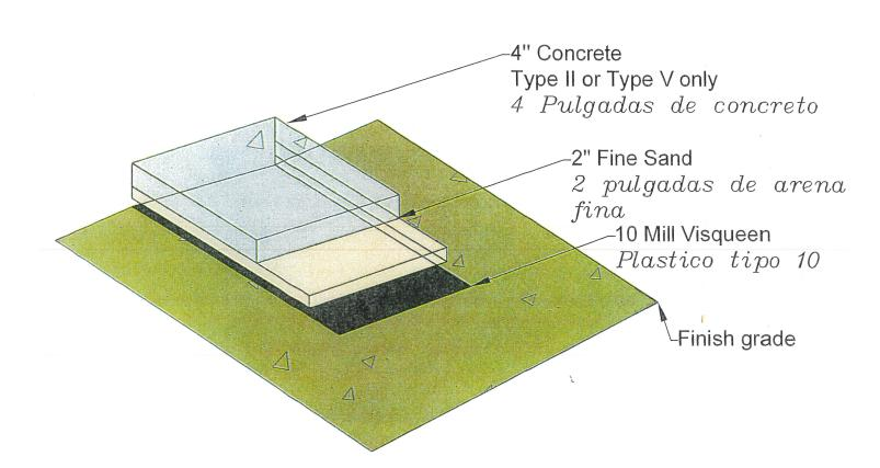
This installation is required due to high sulphate content in the Coachella Valley. Installation of concrete directly on soil or of natural cements will result in accelerated deterioration.
